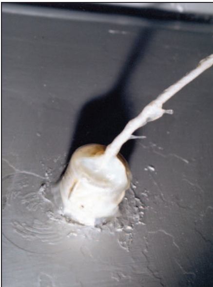
Fig. 109: Closeup of where monitoring line enters chamber also coated in Vaseline.
